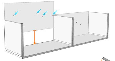
Slide the back(s) into the grooves in the bottom and side panels. Take into account the positions of the openings for the perches and the nesting tray if present (see 🗸 , these must correspond with the front panel, which is still to be installed).
