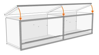
Install the top panel (or the connecting panel) by holding it at an angle and inserting the side panels into the profiles. Lower the top panel onto the base, ensuring that the top edge of the back slides into the groove in the underside of the top panel. Press/tap everything tightly together.
